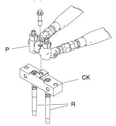
The Fusion AP gun manifold is shown.
