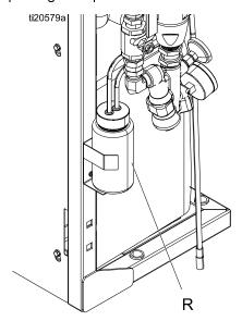
Pump Lubrication System Figure 16
