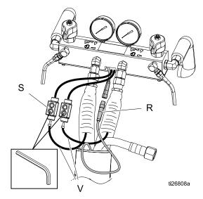
Figure 12 Electrical Splice Connectors
