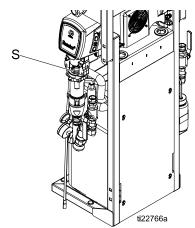
Figure 10 Component B Pump
