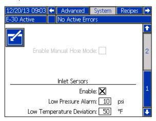
Manual hose mode is automatically disabled when the system detects a valid RTD sensor in the hose.
