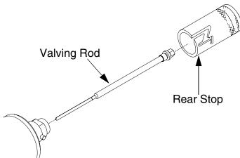
Fig. 25. Remove Valving Rod (GX-7A and GX-7 400 models)
