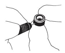
Fig. 29: Clean Module Ports
