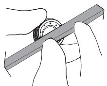
Fig. 28: Unthread Cap from PCD Body
