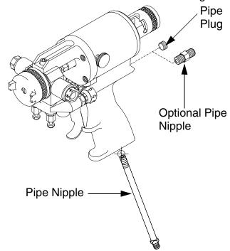
Fig. 16: Air Inlet Configuration
