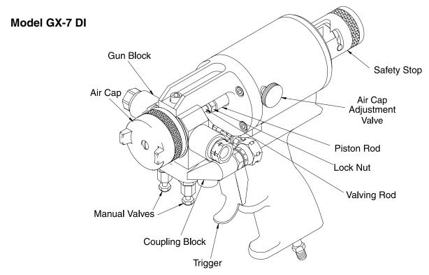
Fig. 2: GX-7 DI Overall View
