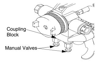
Fig. 14: Open Manual Valves
