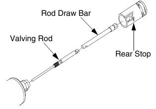
Fig. 24: Remove Valving Rod (GX-7 DI model)
