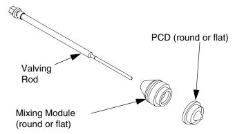
Fig. 7: GX-7A Mixing Module
