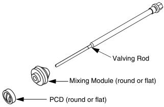
Fig. 8: GX-7 400 Mixing Module
