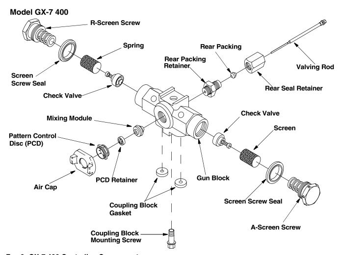
Fig. 6: GX-7 400 Centerline Components
