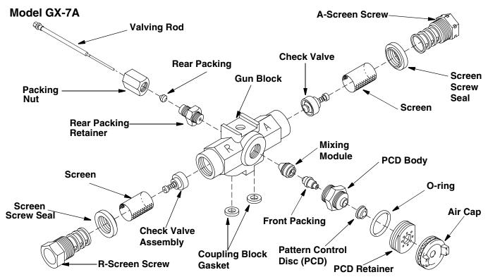
Fig. 4: GX-7A Centerline Components
