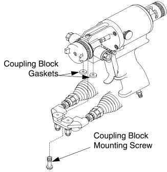
Fig. 15: Install Coupling Block
