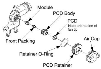
Fig. 30: Install Mixing Module
