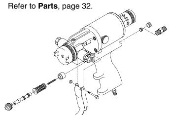
Fig. 27: Replace Trigger Valve O-Ring
