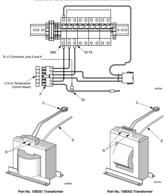
**Detail B: Circuit Breaker Module and Hose Heat Wire Harness**
