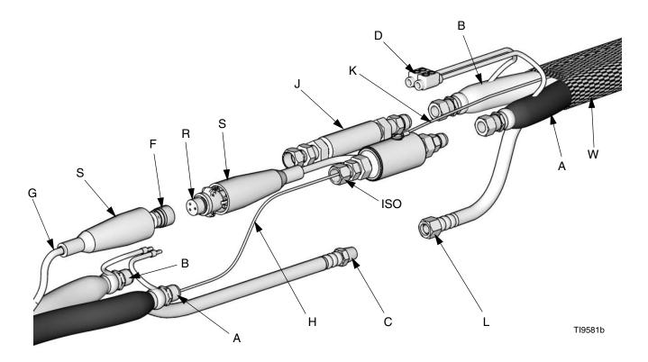
Fig. 12. Fluid Temperature Sensor and Heated Hoses
