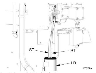
Fig. 17. Pump Lubrication System
