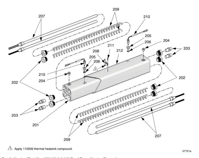
Fig. 9. Heater (Part No. 253189 8.0 kW Dual Zone Heater Shown)
