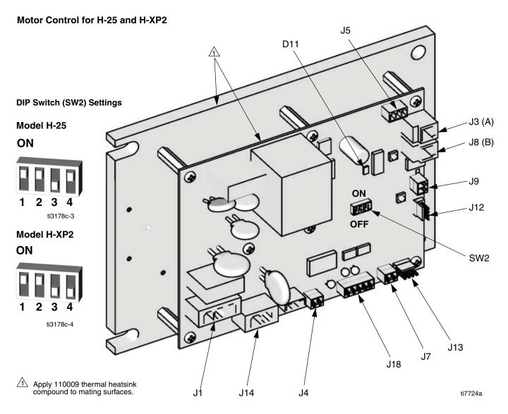
Fig. 4. Motor Control Board
