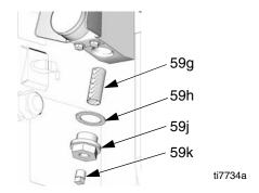
Fig. 16. Y Strainer Components
