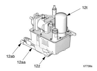
Fig. 18. Change Hydraulic Fluid and Filter
