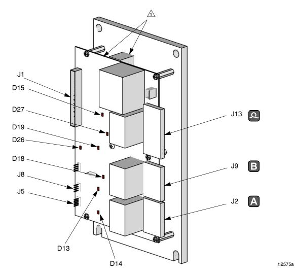
Fig. 8. Temperature Control Board
