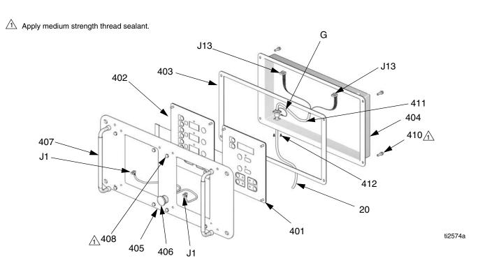
**Detail of Membrane Switches and Display Boards**
